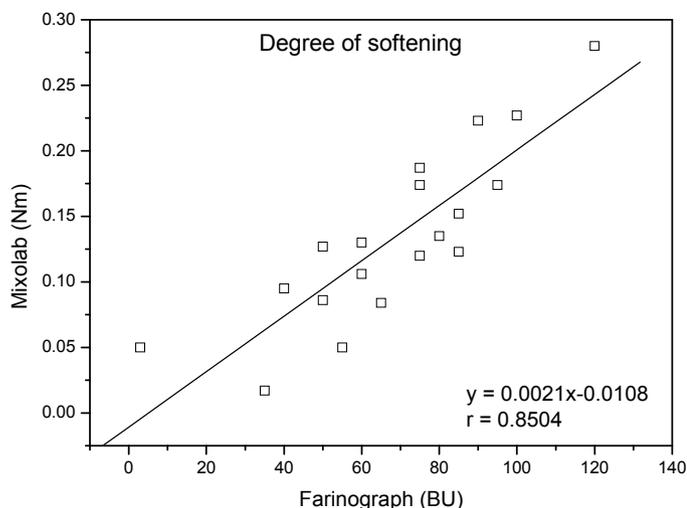
**Figure 6.** Correlation between degree of softening obtained by Mixolab and Farinograph
