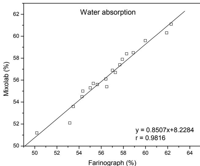
**Figure 3.** Correlation between water absorption obtained by Mixolab and Farinograph
