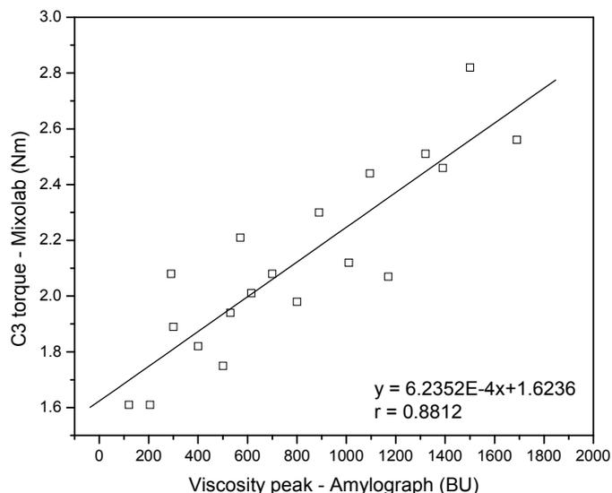
**Figure 7.** Correlation between peak viscosity (Amylograph) and maximum torque during the period of heating (Mixolab)
