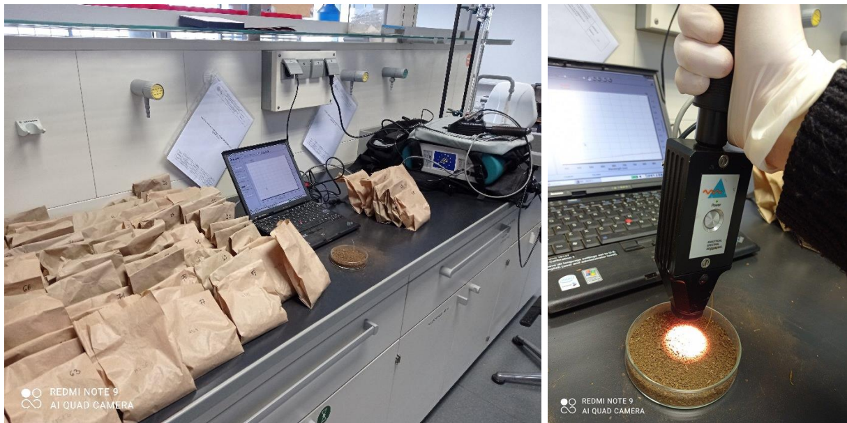
Figure 3.6. Laboratory measurement of soil reflectance on air dried samples using FieldSpec®3 spectroradiometer
