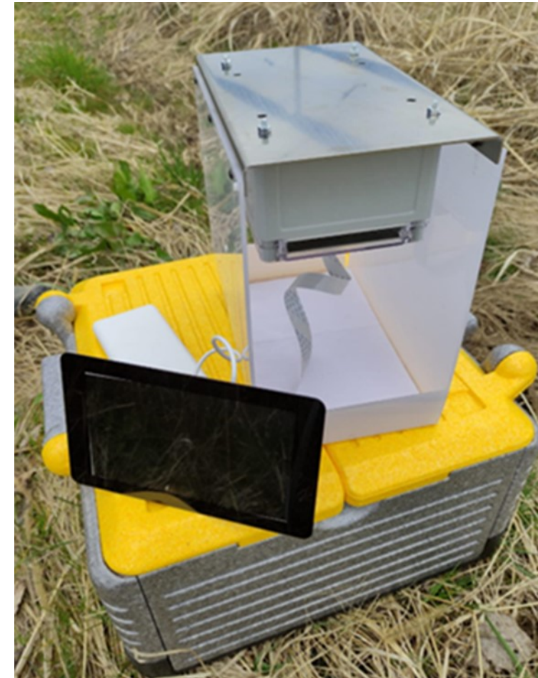
RGB camera in a housing that mimics the prototype of a smart trap for taking photos of adhesive pads
